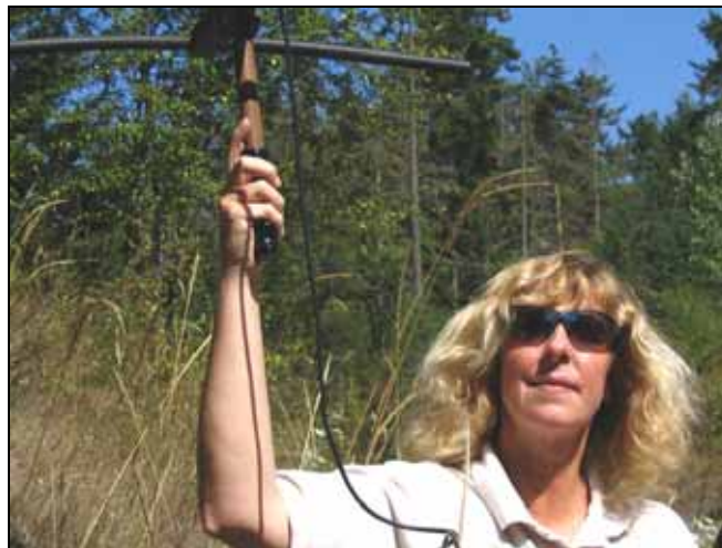
Figure 4.24: Shelly Ament manually scans the frequencies of the radio collared elk in Sequim, Washington, USA (Photo: Marcel Huijser, WTI-MSU)
